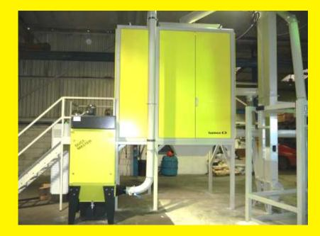
The KWS recovers the finest metallic particles in a dry separation process with a low running cost. Due to its working principle all kinds of non-ferrous metals like copper, aluminium and even rare earth and precious metals are separated from plastics and other non-conductive materials. For best performance the material must be dry and < 5 mm.
